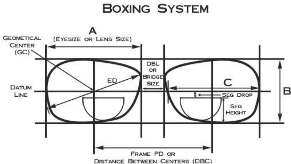
**"A" Measurement** - The horizontal distance between the furthest temporal and nasal edges of the lens shape or the distance between the vertical sides of the box. The A measurement is also commonly known as the **eye size**.
